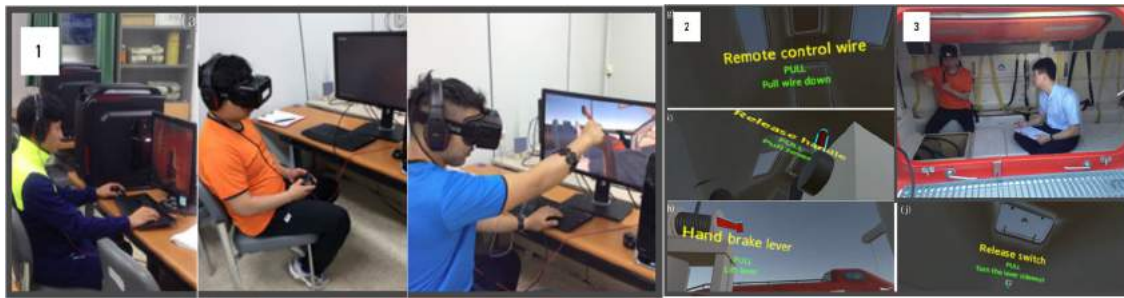
Figure 5. Virtual training interfaces used in the experiment are shown: (a) monitor, keyboard and mouse, (b) head-mounted display and joy pad, (c) head-mounted display and wearable sensors. 2 is the sequential screenshots of the virtual training with guiding instructions. 3 is the evaluation of the VR training later in a real lifeboat [20].
