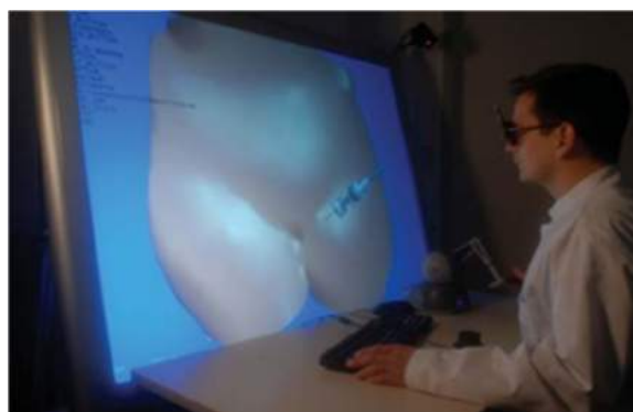
Figure 1. Picture representing RA 1 simulator application with VR based setup. The trainee controls the virtual needle using a PHANTOM Omni Haptic device 2 [10].
