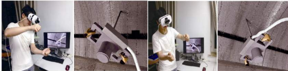
Figure 2. Picture representing RA simulator application with VR based setup. The trainee controls the virtual needle using a PHANTOM Omni Haptic device [13].
